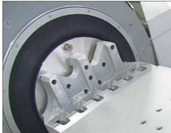
Driver bar is integrally molded with aluminium alloy casting provides a more rigid attachment than welded driver bars. Cast construction has more flexibility, so it can form a rigid and high reliability shape. Welded construction has associated inherent weakness root cracks or blow holes, high quality casting material can eliminate those problem. Bolting line which connects drive bars has the same direction with excitation direction, it is a strong layout for connection.
